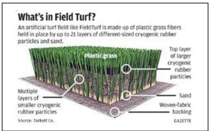
This graphic shows a typical multilayered structure. Plastic grass "blades" (ingredients historically included lead) attach to a fabric backing, separated by an "infill" (usually the tire "crumbs," and sometimes sand). Below them are stones through which drainage pipes go. The infill provides "give." From cdn3.vox-cdn.com/assets/4335789/turfjgraphic.jpg.
